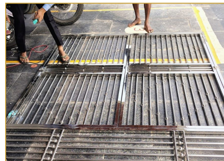
In-house fabrication of SS gate
